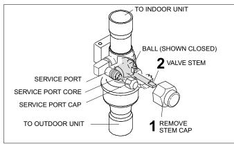
Figure 2. Operating Ball-Type Service Valve ANGLE-TYPE SERVICE VALVE
